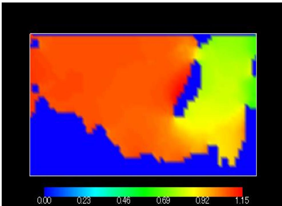
Figure 3 Water level at the time of high tide when the speed of west wind is set as 26m/s
