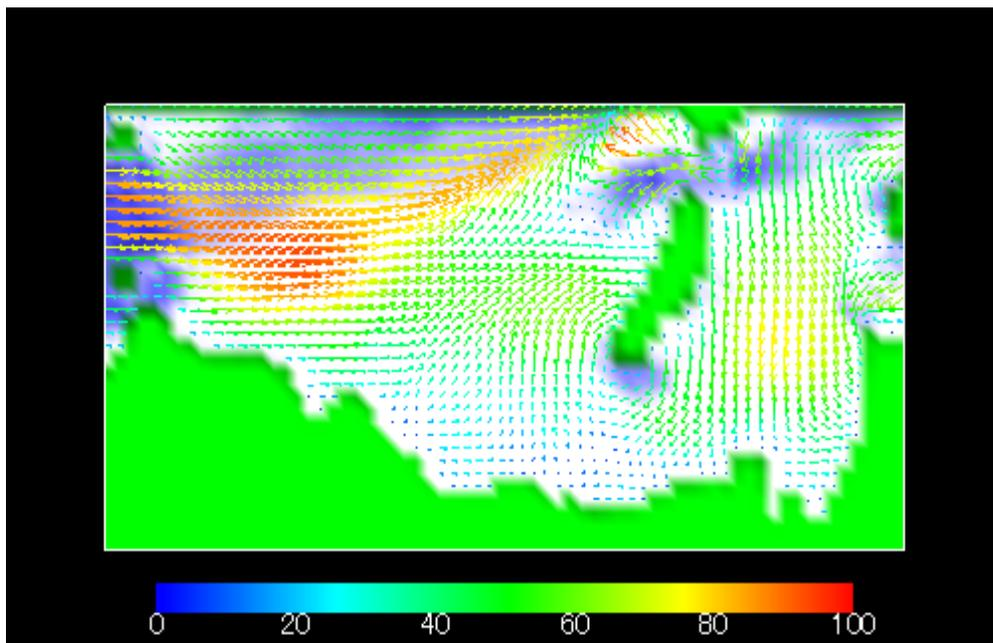
Figure 2 Simulation of tidal current of Takamatsu port area (flood tide against west wind is set as 26m/s)
