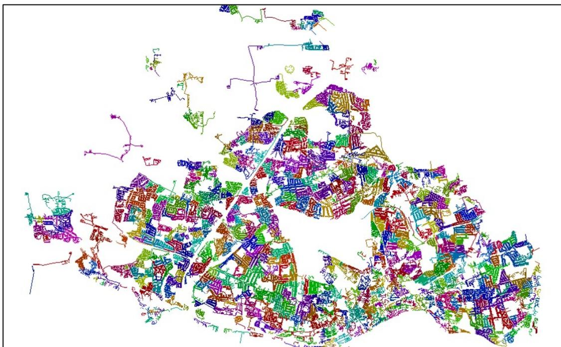
**Figure 3:** Low-voltage electricity distribution network for Newcastle-Upon-Tyne (Contains Ordnance Survey data, Crown copyright 2017).
