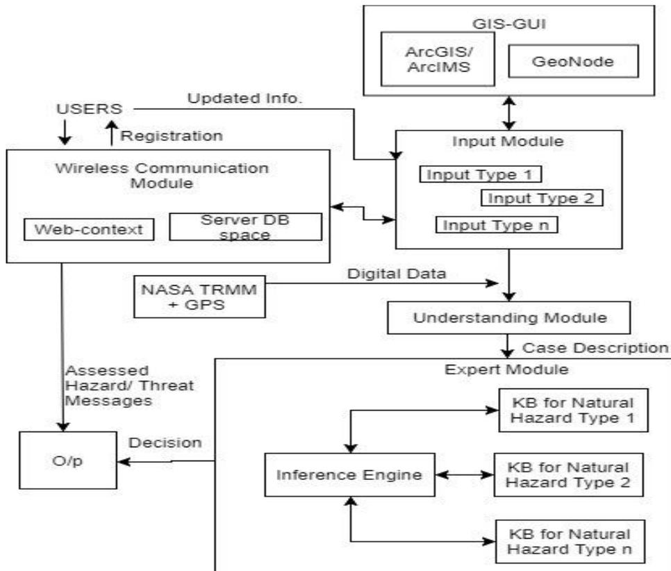
**Figure 1** Schema SmaCiSENS modular architecture & data flow.
